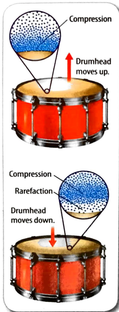
▲ Figure 2 Vibrations of the drumhead produce sound waves.
